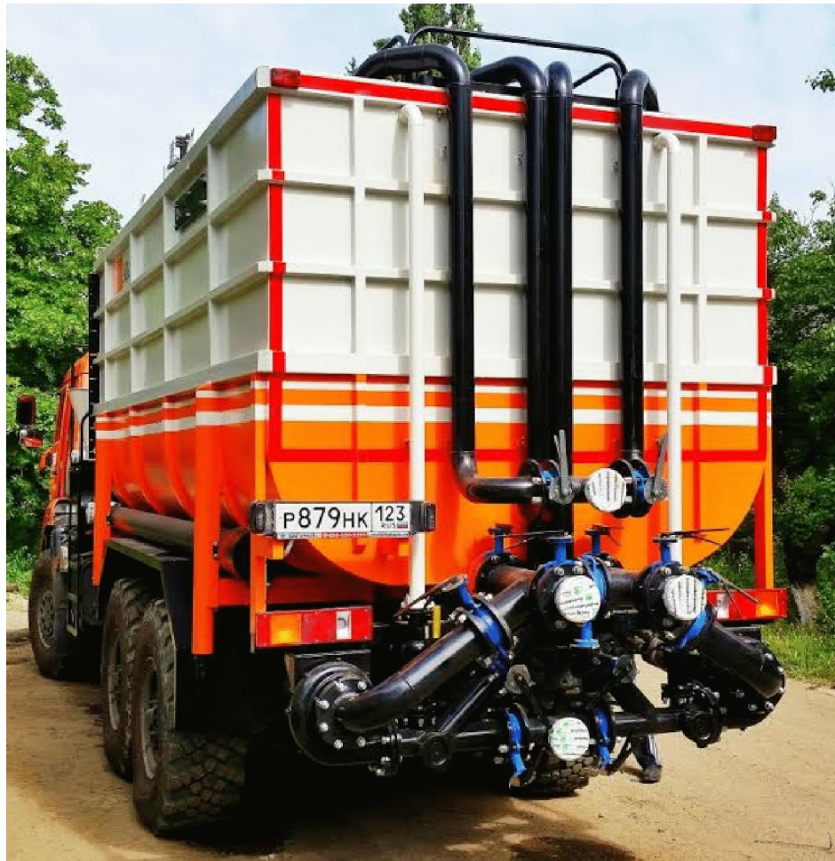
Figure 6 - Mixing surge plant USO-20R1-12
